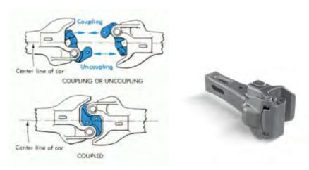
2. **Knuckles:** The pivoting hook-like casting that fits into the head of a coupler and rotates about a vertical pin to either the open position or to the closed position. Knuckles form interlocking pairs within the coupler system that close automatically when freight railcars come together.<sup>17</sup>
